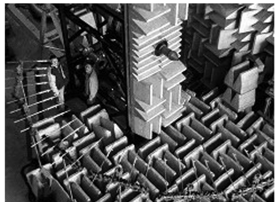
Fig. 2 The SHJAR viewed from above. The 24 microphone array is located on a 100 in. radius, covering angles 15^\circ < \theta < 130^\circ ; \theta is referenced to the downstream jet axis. The nozzle and microphones are eight feet above the wedge tips.
